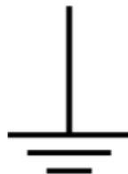
Figure 8: Earthing symbol according to IEC 60417
